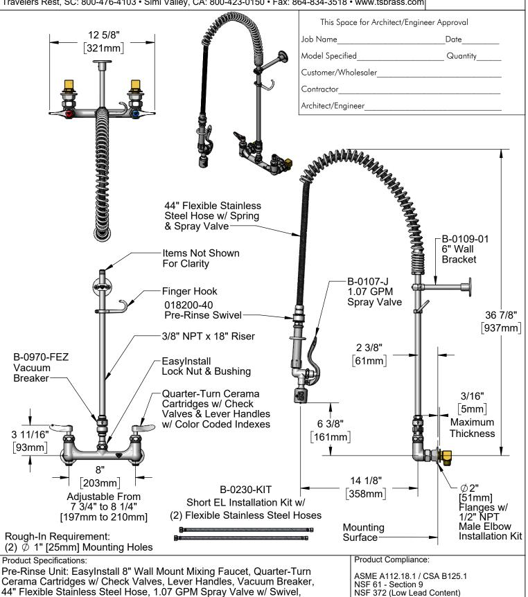
44" Flexible Stainless Steel Hose, 1.07 GPM Spray Valve w/ Swivel,
