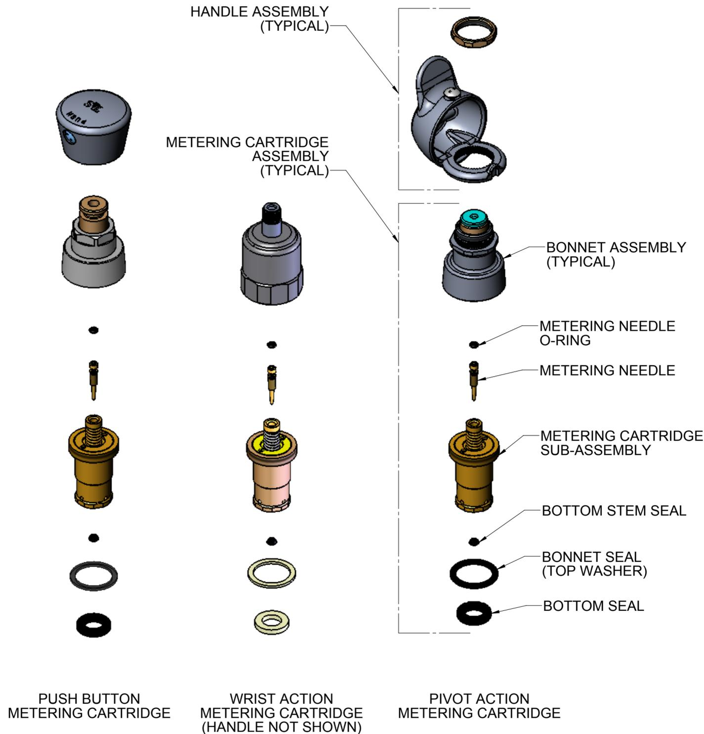
To Replace METERING CARTRIDGE ASSEMBLY Seals:
