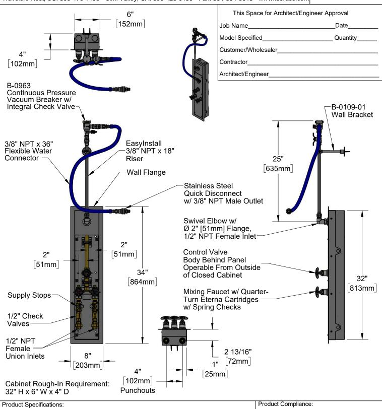
EasyInstall Hose Reel Recess Mounted Cabinet, Concealed Bypass Mixing Valve, Eterna Cartridges w/ Spring Checks, Loose-Key Supply Stops, 1/2" NPT Female Union Inlets, Control Valve w/ Eterna Cartridge, 1/2" NPT Riser, Check Valves, Swivel Elbows w/ 1/2" NPT Female Inlet, EasyInstall 3/8" NPT x 18" Riser, 6" Wall Bracket, Continuous Pressure Vac. Breaker w/ Integral Check Valve, Removable Wall Flange, 36" Flexible Water Hose w/ Stainless Steel Quick Disconnect & 3/8" NPT Male Outlet
