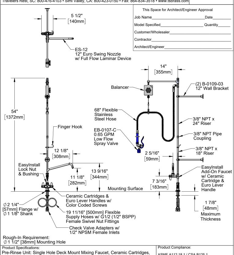
Pre-Rinse Unit: Single Hole Deck Mount Mixing Faucet, Ceramic Cartridges, Euro Lever Handles, Add-On Faucet w/ 12" Swing Nozzle, 68" Flexible Stainless Steel Hose, 0.65 GPM Low Flow Spray Valve, Balancer, Extension Arm, (2) 12" Wall Brackets, 19 11/16" [500mm] Flexible Supply Hoses w/ G1/2 (1/2" BSPP) Female Nut Fittings & Check Valve w/ 1/2" NPSM Female Inlets
