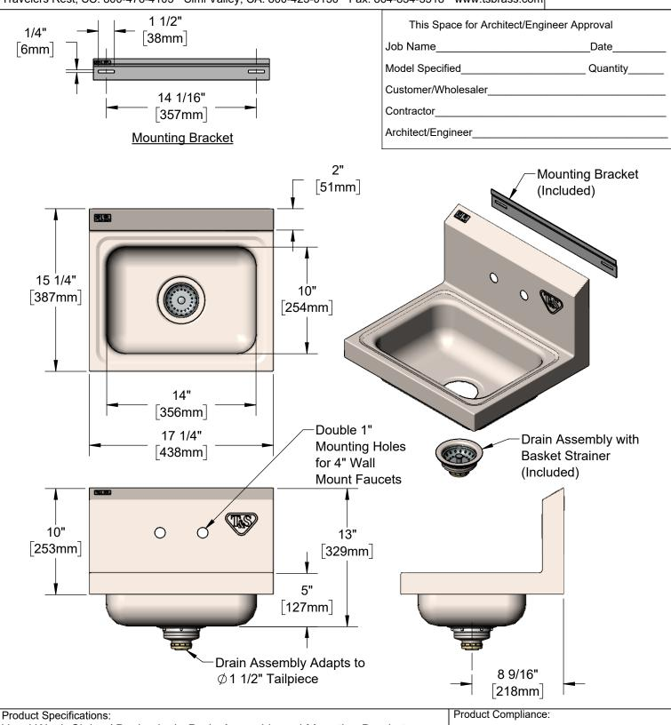
Hand Wash Sink w/ Backsplash, Drain Assembly and Mounting Bracket, NSF Approved, Stainless Steel, 17" x 15" Overall, 14" x 10" Bowl, 4" c/c Faucet Mounting Holes, 3 1/2" Drain Hole
