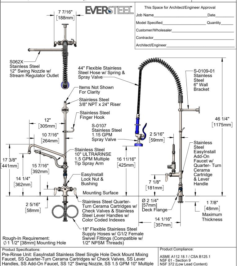
Tip Spray Arm, 44" Flexible Stainless Steel Hose, SS 1.15 GPM Spray Valve,
