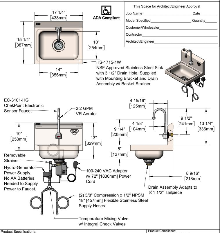
Hand Wash Sink / Elec. Sensor Faucet, Stainless Steel Sink / Backsplash, 3 1/2" Drain Assembly, Electronic Sensor Faucet, Wall Mount Rigid Gooseneck w/ 2.2 GPM VR Aerator, AC/DC Control Module w/ Internal Flow Cont. Setting Switches, Temperature Control Mixing Valve w/ Check Valves, Hydro-Generator 18" Hot & Cold Supply Stop Flexible Connector Hoses
