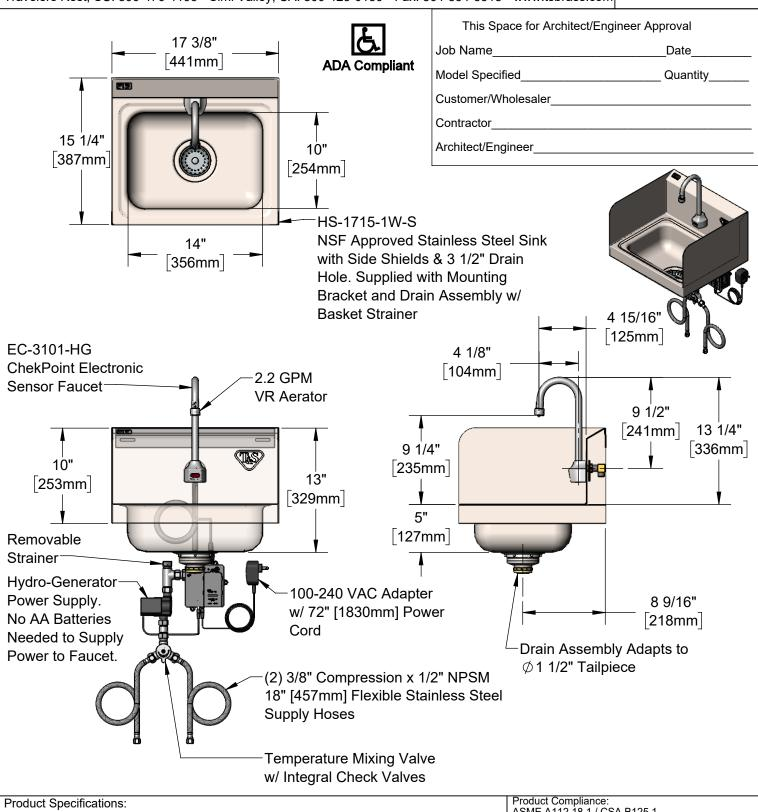
Hand Wash Sink / Elec. Sensor Faucet, Stainless Steel Sink / Backsplash, Side Splash Shields, 3 1/2" Drain Assembly, Electronic Sensor Faucet, Wall Mount Rigid Gooseneck w/ 2.2 GPM VR Aerator, AC/DC Control Module w/ Internal Flow Cont. Setting Switches, Temperature Control Mixing Valve w/ Check Valves, Hydro-Generator 18" Hot & Cold Supply Stop Flexible Connector Hoses
