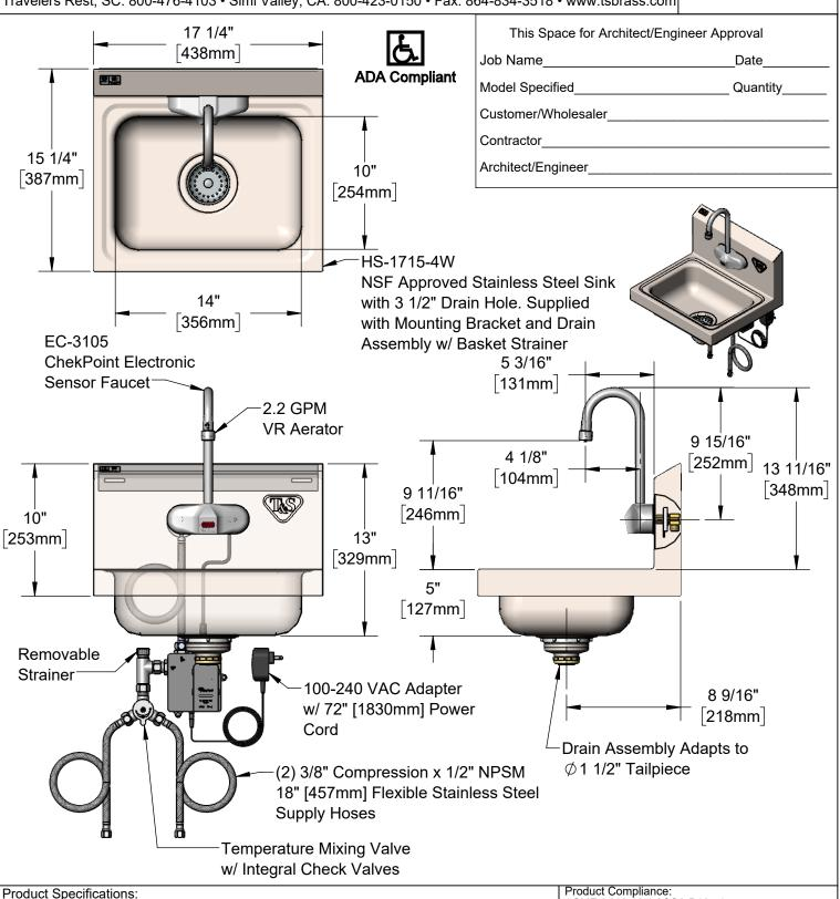
Hand Wash Sink / Elec. Sensor Faucet, Stainless Steel Sink / Backsplash, 3 1/2" Drain Assembly, Electronic Sensor Faucet, 4" c/c Wall Mount Rigid Goosneck w/ 2.2 GPM VR Aerator, AC/DC Control Module w/ Internal Flow Control Setting Switches, Temperature Control Mixing Valve w/ Check Valves, 18" Flexible Stainless Steel Supply Hoses
