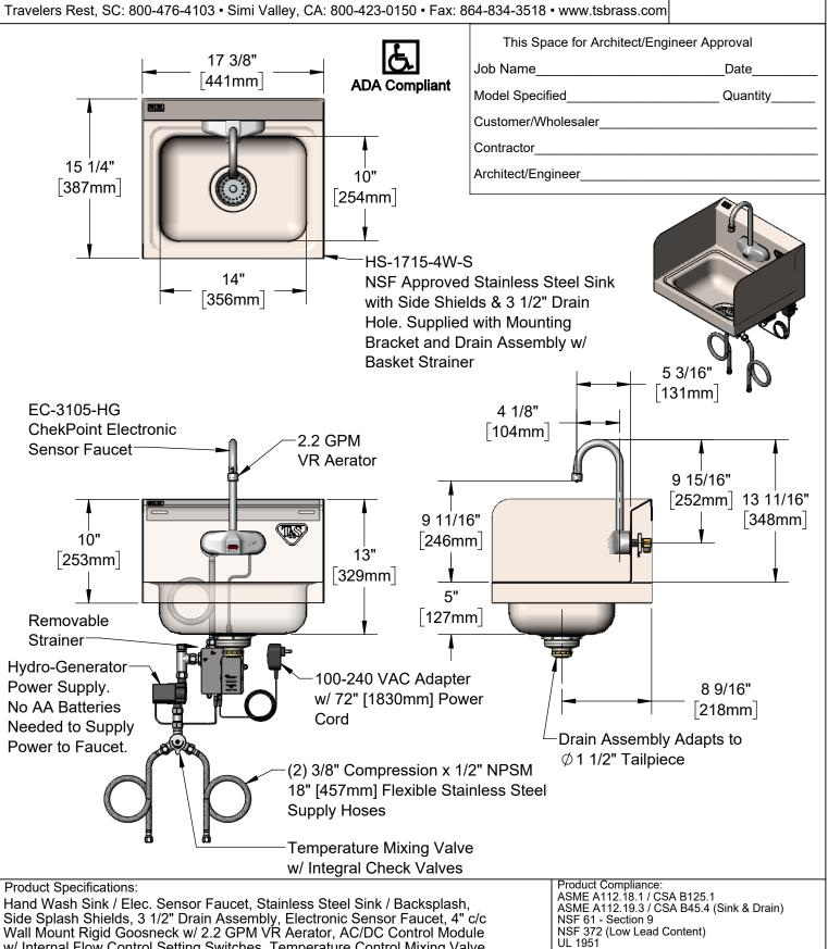
w/ Internal Flow Control Setting Switches, Temperature Control Mixing Valve w/ Check Valves, Hydro Generator & 18" Flexible Stainless Steel Supply
