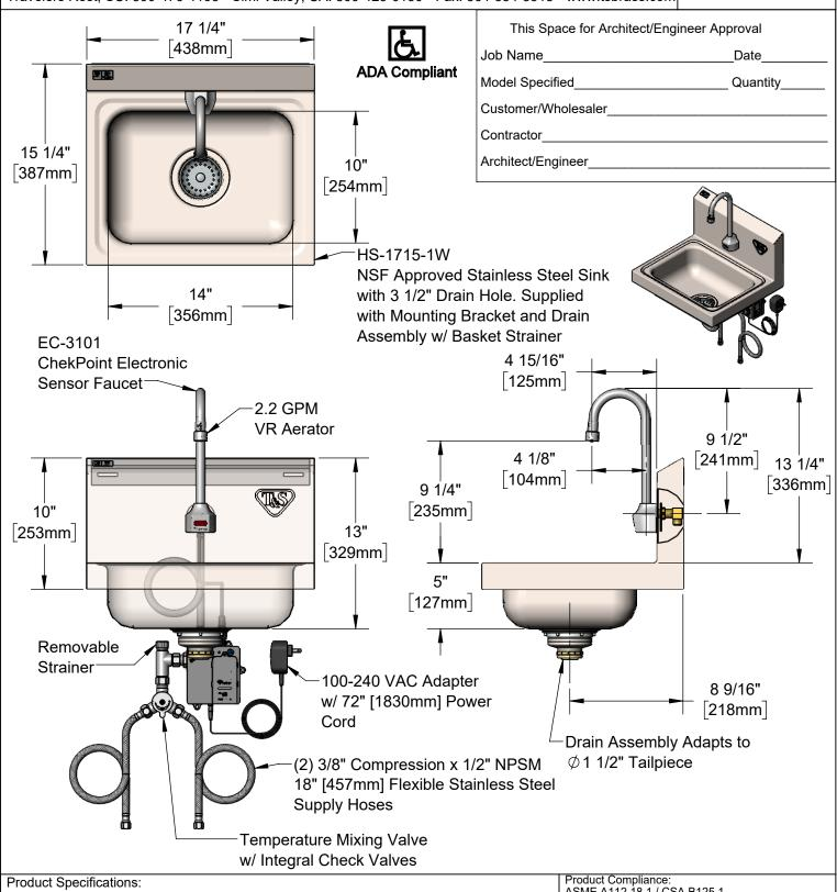
Hand Wash Sink / Elec. Sensor Faucet, Stainless Steel Sink / Backsplash, 3 1/2" Drain Assembly, Electronic Sensor Faucet, Wall Mount Rigid Gooseneck w/ 2.2 GPM VR Aerator, AC/DC Control Module w/ Internal Flow Control Setting Switches, Temperature Control Mixing Valve w/ Check Valve, 18" Hot & Cold Supply Stop Flexible Connector Hoses
