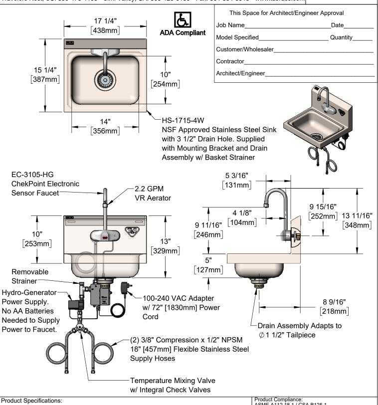
Hand Wash Sink / Elec. Sensor Faucet, Stainless Steel Sink / Backsplash, 3 1/2" Drain Assembly, Electronic Sensor Faucet, 4" c/c Wall Mount Rigid Goosneck w/ 2.2 GPM VR Aerator, AC/DC Control Module w/ Internal Flow Control Setting Switches, Temperature Control Mixing Valve w/ Check Valves, Hydro Generator & 18" Flexible Stainless Steel Supply Hoses
