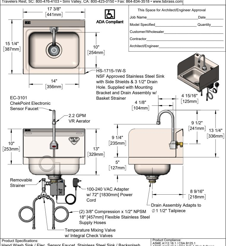
Hand Wash Sink / Elec. Sensor Faucet, Stainless Steel Sink / Backsplash, Side Splash Shields, 3 1/2" Drain Assembly, Electronic Sensor Faucet, Wall Mount Rigid Gooseneck w/ 2.2 GPM VR Aerator, AC/DC Control Module w/ Internal Flow Control Setting Switches, Temperature Control Mixing Valve w/ Check Valve, 18" Hot & Cold Supply Stop Flexible Connector Hoses
