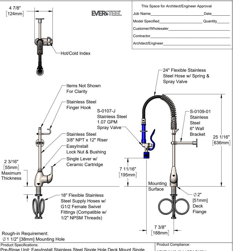
Pre-Rinse Unit: EasyInstall Stainless Steel Single Hole Deck Mount Single Lever Faucet, Ceramic Cartridge, 24" Flexible Stainless Steel Hose, Stainless Steel 1.07 GPM Spray Valve, Stainless Steel 6" Wall Bracket & Flexible Stainless Steel Supply Hoses
