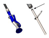
Step 2: For Pre-Rinse Units: apply plumber's tape to top of riser threads and attach to spring assembly. Tighten with wrench.
