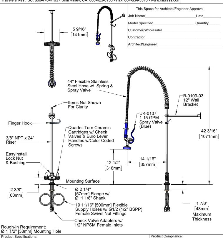
Pre-Rinse Unit: Single Hole Deck Mount Mixing Faucet, Ceramic Cartridges w/ Check Valves, Euro Lever Handle, 1.15 GPM Spray Valve (Blue), 44" Flexible Stainless Steel Hose, 12" Wall Bracket, 19 11/16" [500mm] Flexible Supply Hoses w/ G1/2 (1/2" BSPP) Female Nut Fittings & Check Valve Adapters w/ 1/2" NPSM Female Inlets
