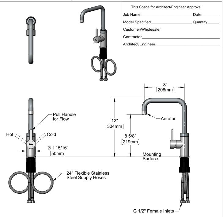
Rough-In Requiement:  $\emptyset$  1 1/2" [38mm] Mounting Hole
