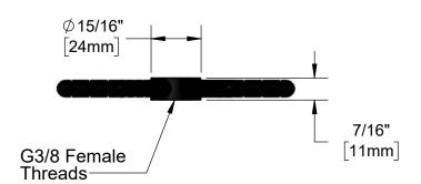
Product Compliance: Product Specifications: Star Bracket Replacement Part for EX-RINSERS Drawn: KJG Checked: MRC Approved: JHB Date: 07/30/19 Scale: 1:2 Sheet: 1 of 1
