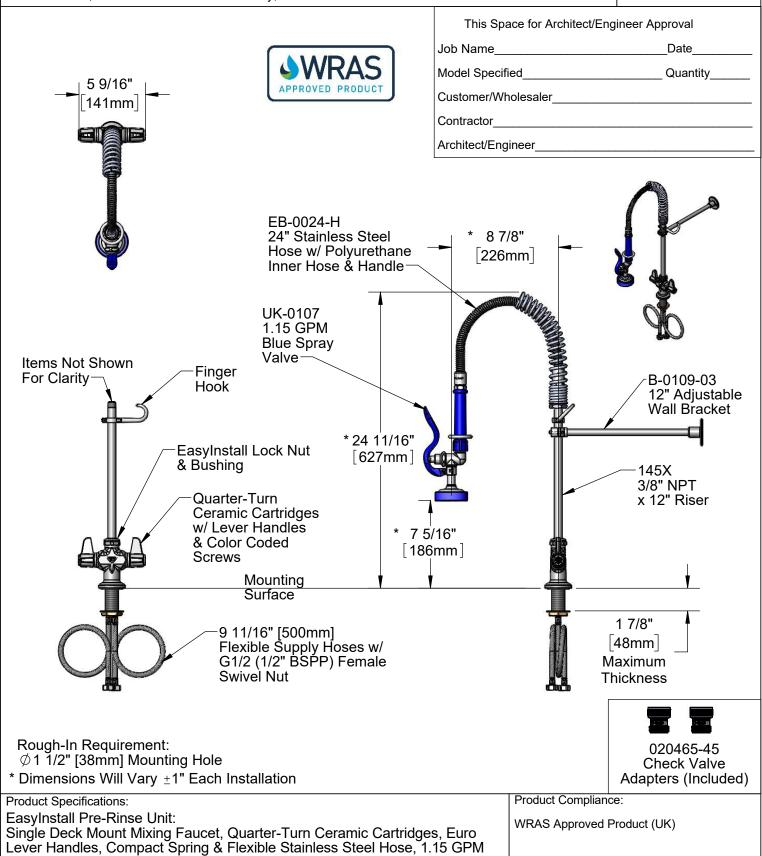
Spray Valve (Blue), 12" Wall Bracket & 19 11/16" Flexible Hoses w/ G1/2
