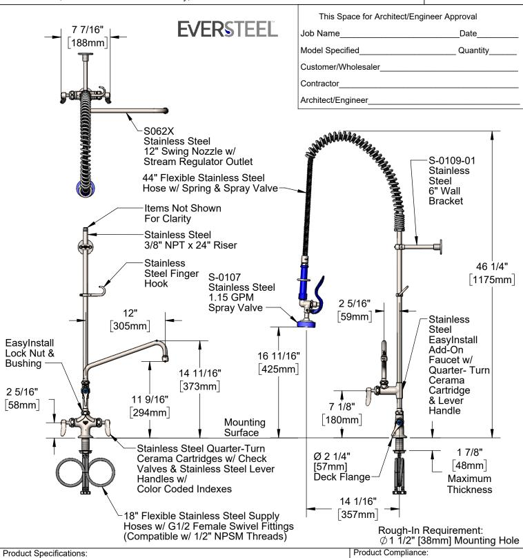
Pre-Rinse Unit: EasyInstall Stainless Steel Single Hole Deck Mount Mixing Faucet, SS Quarter-Turn Cerama Cartridges w/ Check Valves, SS Lever Handles, SS Add-On Faucet, SS 12" Swing Nozzle, 44" Flexible Stainless Steel Hose, SS 1.15 GPM Spray Valve, SS 6" Wall Bracket & Flexible Stainless Steel Supply Hoses
