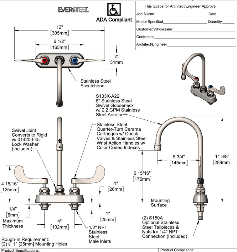
4" Stainless Steel Deck Mount Workboard Faucet, Stainless Steel Quarter-Turn Cerama Cartridges w/ Check Valves, 4" Stainless Steel Wrist Action Handles, 6" Stainless Steel Swivel Gooseneck, 2.2 GPM Stainless Steel Aerator & 1/2" NPT Stainless Steel Male Inlets
