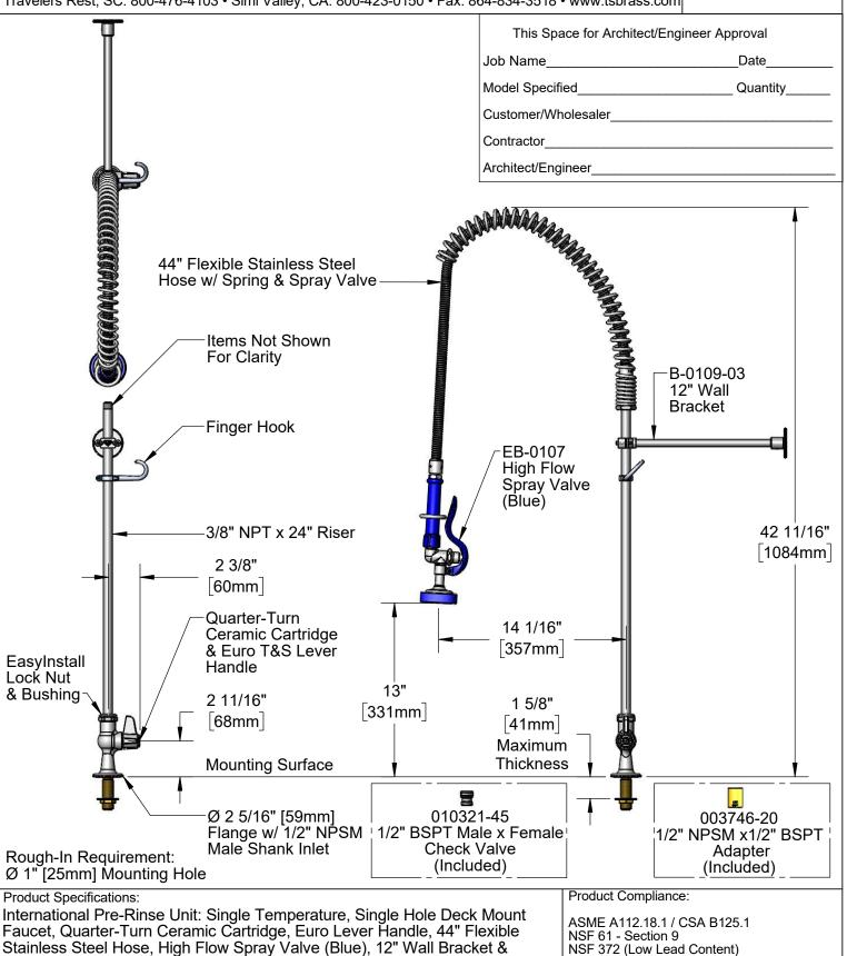
1/2" NPSM Shank Inlet w/ BSPT Adapter & Check Valve
