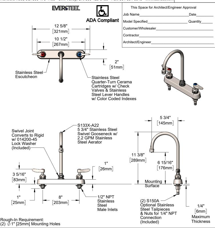
8" Stainless Steel Deck Mount Workboard Faucet, Stainless Steel Quarter-Turn Cerama Cartridges w/ Check Valves, Stainless Steel Lever Handles, 5 3/4" Stainless Steel Swivel Gooseneck, 2.2 GPM Stainless Steel Aerator & 1/2" NPT Stainless Steel Male Inlets Product Compliance:
