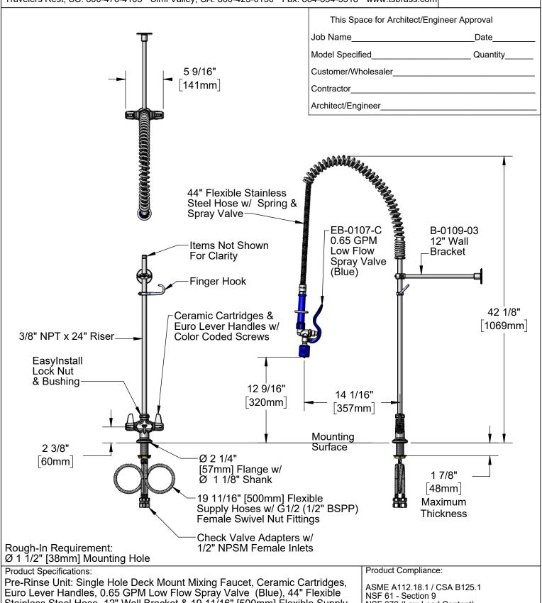
Stainless Steel Hose, 12" Wall Bracket & 19 11/16" [500mm] Flexible Supply Hoses w/ G1/2 (1/2" BSPP) Female Nut Fittings & Check Valve Adapters w/ 1/2" NPSM Female Inlets
