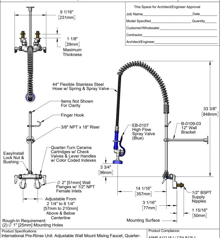
International Pre-Rinse Unit: Adjustable Wall Mount Mixing Faucet, Quarter-Turn Cerama Cartridges w/ Check Valves, Lever Handles, 44" Flexible Stainless Steel Hose, High Flow Spray Valve (Blue), 12" Wall Bracket & 1/2" NPT Female Adjustable Arm Inlet Flanges w/ 1/2" BSPT Male Supply Kit ASME A112.18.1 / CSA B125.1 NSF 61 - Section 9 NSF 372 (Low Lead Content) 2019 DOE PRSV Non-Compliant Product Not Designed/Intended for Commercial Warewashing in North America
