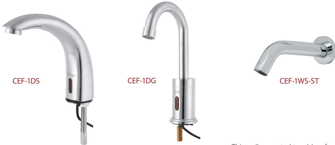
The CEF-1D series sensor faucets are single-hole, dual temperature, deck-mounted and come with vandal-resistant 8.3 L/min (2.2 GPM) aerators (unless otherwise stated), AC/DC transformers, control modules, mechanical mixing valves, G 1/2" flexible supply hoses and G 3/8" adapters. They can also run on batteries as a stand-alone solution.
