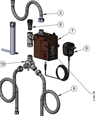
A Maximum of (8) ChekPoint Faucets can be Hardwire Connected and Powered by EC-HARDWIRE ChekPoint Hardwire AĆ Transformer. (Sold Separately)
