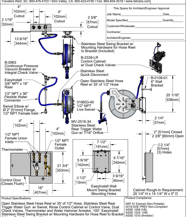
Stainless Steel Swing Bracket w/ Mounting Hardware for Hose Reel to Bracket
