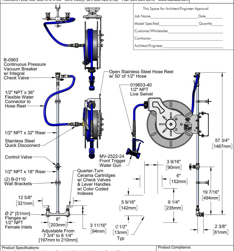
Open Stainless Steel Hose Reel w/ 50' of 1/2" Hose, Front Trigger Water Gun w/ Swivel, 1/2" NPT Vacuum Breaker, 1/2" NPT Flexible Water Connector, 8" Wall Mount Mixing Faucet, Control Valve & EasyInstall Wall Swing Bracket
