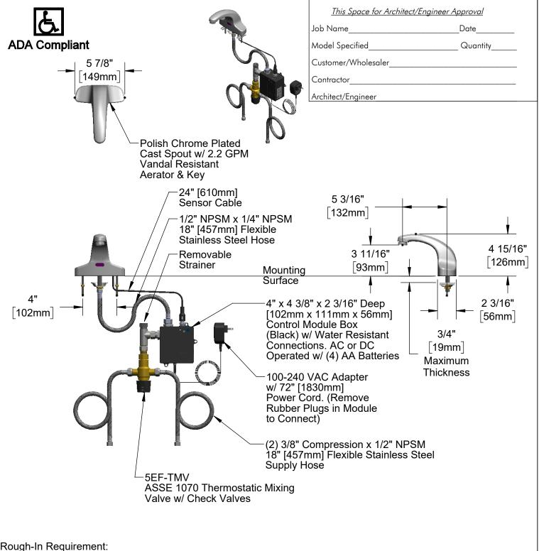
(1)  $\emptyset$  1" [25mm] Center Shank Mounting Hole & (2)  $\emptyset$  1/2" [13mm] Mounting Stud Holes on 4" [102mm] Centers
