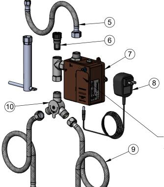
A Maximum of (8) ChekPoint Faucets can be Hardwire Connected and Powered by EC-HARDWIRE ChekPoint Hardwire AĆ Transformer. (Sold Separately)
