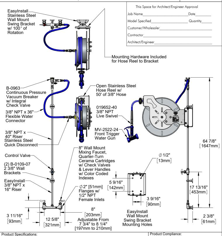
Open Stainless Steel Hose Reel w/ 50' of 3/8" Hose, Blue Front Trigger Water Gun w/ Swivel, Vacuum Breaker, 3/8" NPT Flexible Water Connector, 8" Wall Mount Mixing Faucet w/ Quarter-Turn Cerama Cartridges & Lever Handles, Control Valve, 100 Degree EasyInstall Stainless Steel Swing Bracket w/ Mounting Hardware for Hose Reel to Bracket
