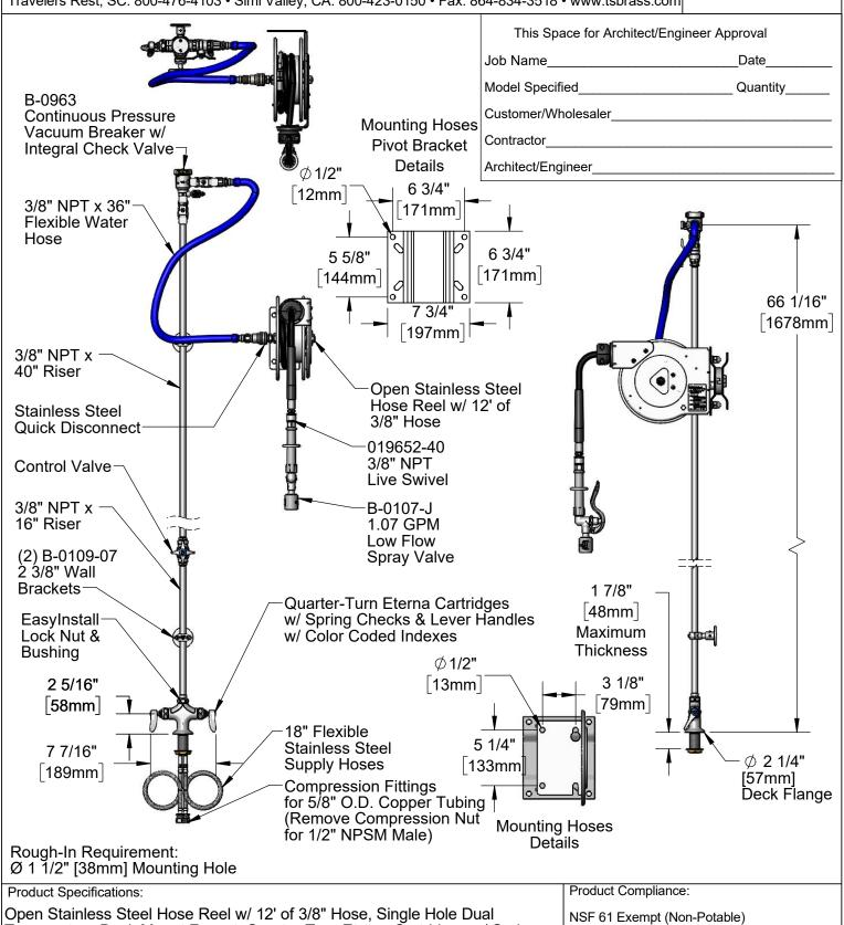
Open Stainless Steel Hose Reel w/ 12' of 3/8" Hose, Single Hole Dual Temperature Deck Mount Faucet, Quarter-Turn Eterna Cartridges w/ Spring Checks, 1.07 GPM Low Flow Spray Valve w/ Swivel, Vacuum Breaker, 3/8" NPT Flexible Water Hose, Wall Brackets, 345° Epoxy Coated Pivot Deck Mount Bracket w/ Mounting Hardware for Hose Reel to Bracket & Control Valve
