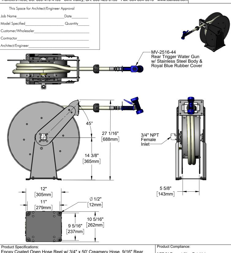
Epoxy Coated Open Hose Reel w/ 3/4" x 50' Creamery Hose, 9/16" Rear Trigger Water Gun & Double Arm Support
