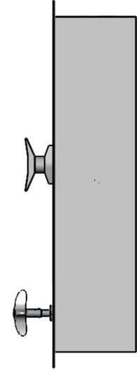
Main Shutoff Valve Body Behind Panel. Handle Is Operable From Outside Of Closed Cabinet
