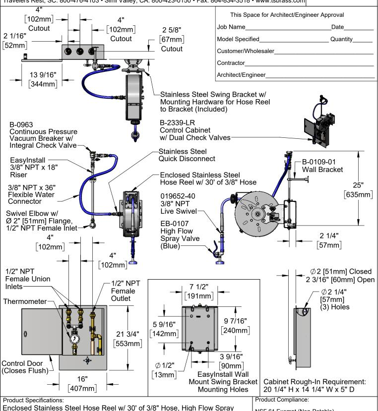
Enclosed Stainless Steel Hose Reel w/ 30' of 3/8" Hose, High Flow Spray Valve (Blue) w/ Swivel, Rinse Control Cabinet w/ Control Valve, Dual Check Valves, Thermometer and Water Hammer Arrestor, 100° EasyInstall Stainless Steel Swing Bracket w/ Mounting Hardware for Hose Reel to Bracket & Hose Reel Connector Kit
