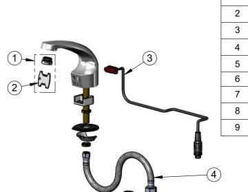
ITEM SALES NO. **DESCRIPTION** NO. 1 B-0199-08 VR 2.2 GPM Aerator, 13/16-27 UN Male w/ Key 015425-45 Vandal Resistant Key 019174-45 Sensor Cable Assembly Inlet Hose, Faucet, 1/2" NPSM-F x 1/4" NPSM-F 016297-45 019944-45 ChekPoint Control Module w/ Filter Tee 5EF-0002C | AC Adapter - US Plug 5EF-0005 Supply Hose, 9/16-24 Female x 1/2" NPSM 5EF-0006 Temperature Mixing Valve EC-FILTER | Replacement Filter
