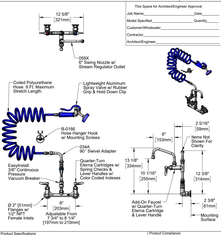
Pet Grooming Station: 8" Wall Mount Mixing Faucet, Quarter-Turn Eterna Cartridges w/ Spring Checks, Lever Handles, Vacuum Breaker, Add-On Faucet, 6" Swing Nozzle w/ Stream Regulator Outlet, 90° Swivel Arm, 9' Coiled Hose w/ Angled Aluminum Spray Valve, Hanger Hook & 1/2" NPT Female Inlets
