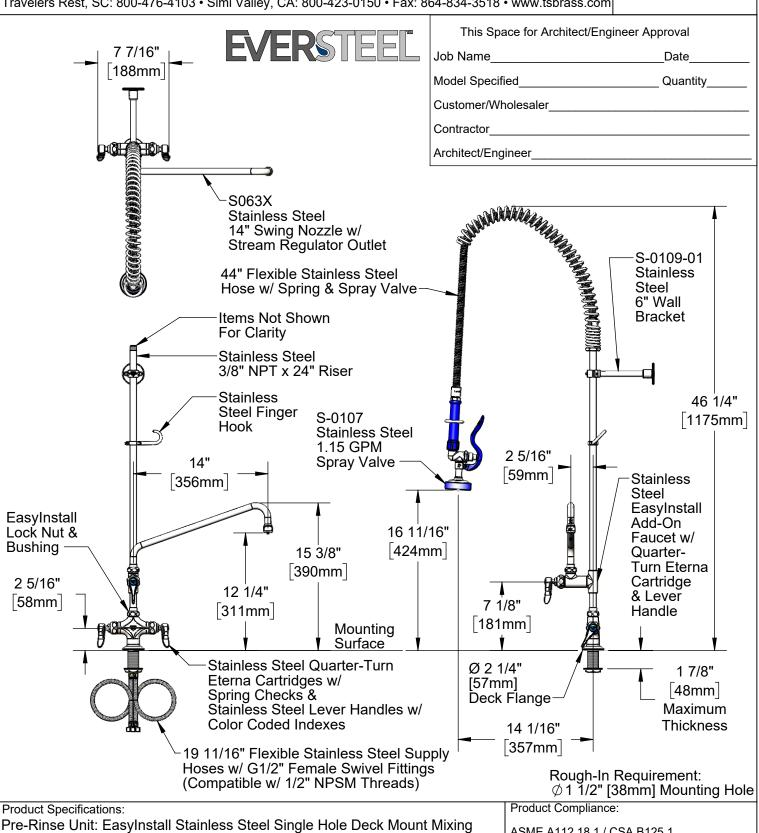
Pre-Rinse Unit: EasyInstall Stainless Steel Single Hole Deck Mount Mixing Faucet, SS Quarter-Turn Eterna Cartridges w/ Spring Checks, SS Lever Handles, SS Add-On Faucet, SS 14" Swing Nozzle, 44" Flexible Stainless Steel Hose, SS 1.15 GPM Spray Valve, SS 6" Wall Bracket & Flexible Stainless Steel Supply Hoses
