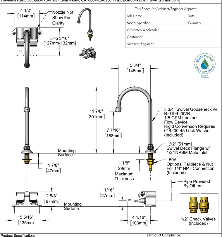
Floor-Mounted Double Pedal Valve w/ 5 3/4" Rigid/Swivel Gooseneck w/ VR 1.5 GPM Laminar Device Outlet
