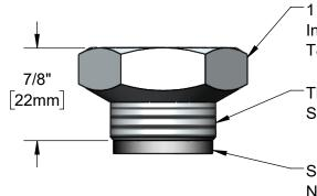
1 3/8" [35mm] Hex with Internal Threads to fit T&S Wall Mount Faucet Body
